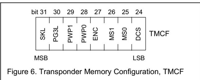
The memory access rights applied by TMCF affect the behavior of READ\_PAGE and WRITE\_PAGE commands only. Device operation, e.g. with respect to the authentication process, is not affected at all.
