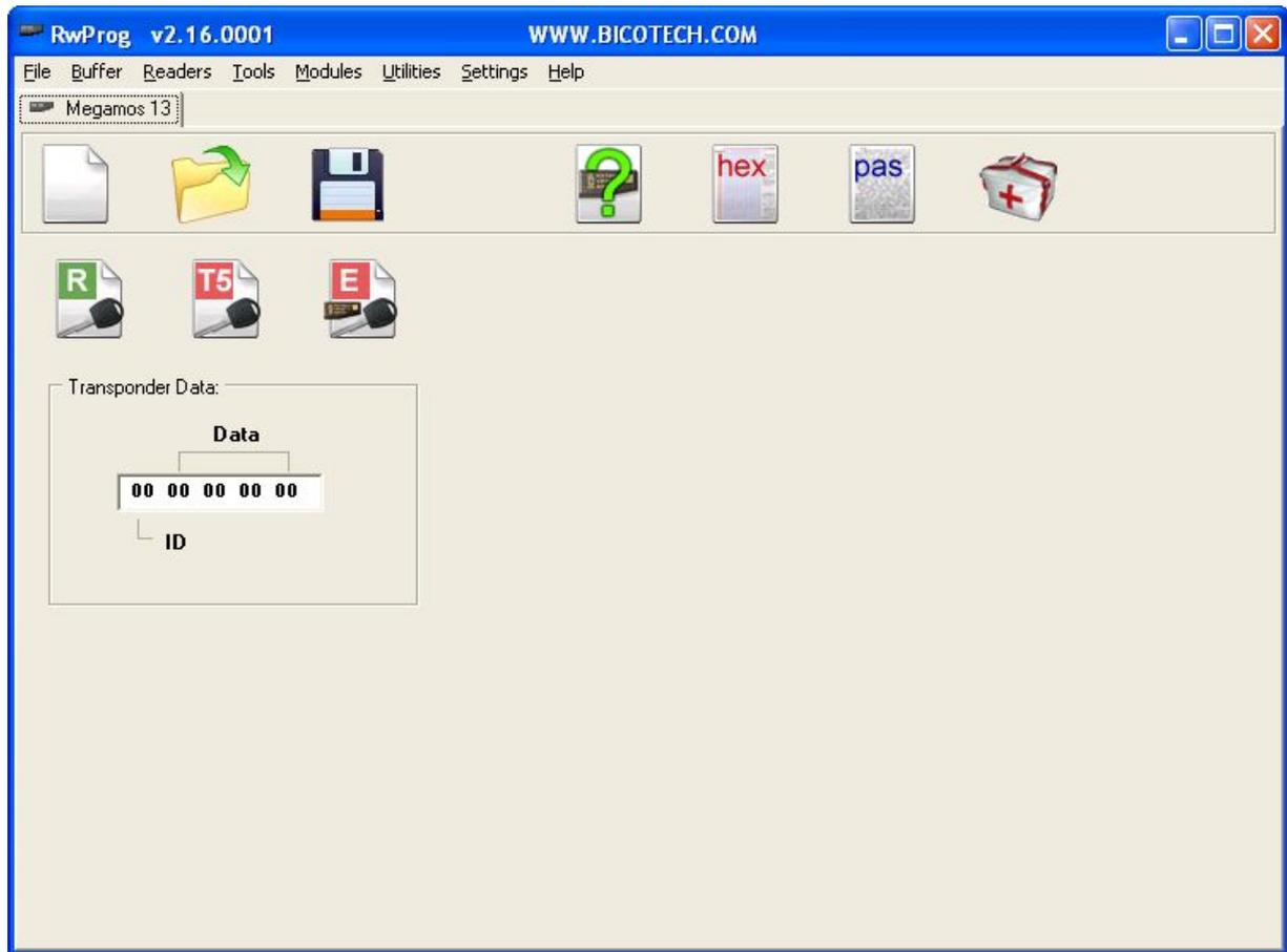
Operation with Megamos ID13 transponders is similar to operation with transponders Temic ID11, ID12 transponders. Difference is displayed data is corresponding to the real transponder data.
